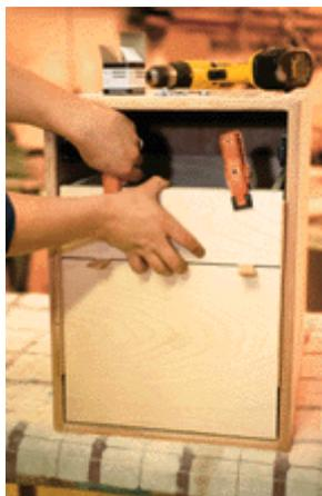
A consistent reveal is key to the crisp feel of the piece. The shims shouldn't bow the cabinet sides out at all, but should fit snugly to ensure that the drawer front is
