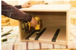
Using spacers to position the drawer slides eliminates one of the leading causes of poor-fitting drawers: inconsistent spacing of slides. Before putting in the spacers, be sure to brush out any sawdust or woodchips that may have accumulated inside the cabinet. A  $\frac{1}{16}$ " discrepancy at this point could cause an annoying misalignment that you'll have to backtrack to correct later on.
